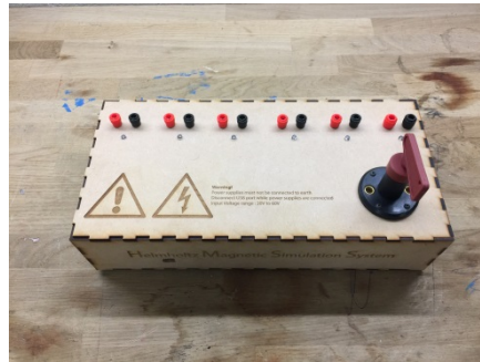
Figure 20: Enclosure for the Helmholtz circuitry
