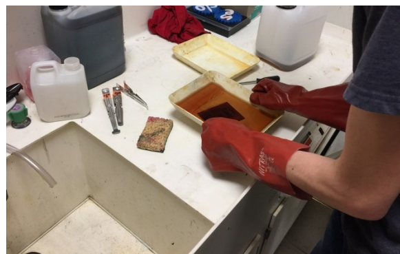
Figure 19: Etching of the logic circuit board
